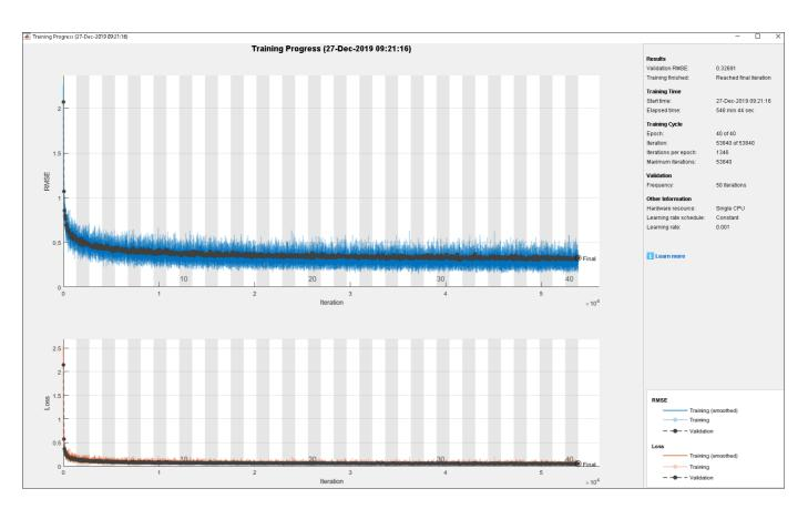
The training of the DNN using behavior cloning reduces the gap between the DNN and NLMPC performance. However, the behavior cloning neural network fails to imitate the behavior of the NLMPC controller correctly on some randomly generated data.
