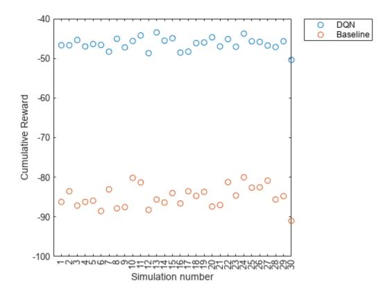
The cumulative reward obtained by the agent is consistently around -40. This value is much greater than the average reward obtained by the baseline controller. Therefore, the DQN agent consistently outperforms the baseline controller in terms of energy savings.
