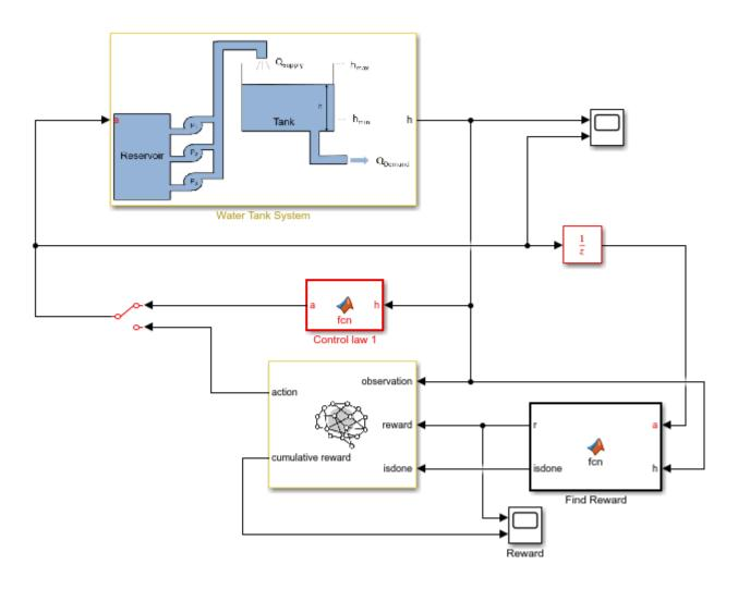
In addition to the reinforcement learning agent, a simple baseline controller is defined in the Control law MATLAB Function block. This controller activates a certain number of pumps depending on the water level.
