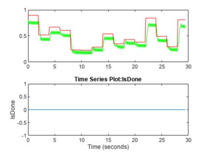
The agent tracks the position of the red ball with more steady-state offset than the agent trained with constraints.
