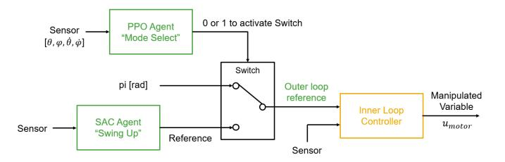
The mode-switching action (0 or 1) switches the outer-loop reference signal between the trajectory generated by the swing-up agent action and  $\pi$  radians.
