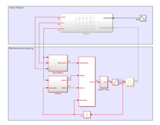
The model contains an RL Agent block with its **last action** input port enabled. This input port allows the specification of custom noise in the Simulink model for off-policy RL agents, such as deep deterministic policy gradient (DDPG) agents.
