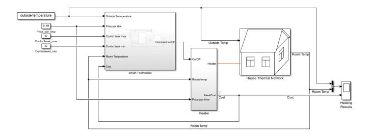
The training goal for the agent is to minimize the energy cost and maximize the comfort of the room by turning on/off the heater. The house is comfortable when the room temperature  $T_{\rm room}$  is between  $T_{\rm comfortMin}$  and  $T_{\rm comfortMax}$ .
