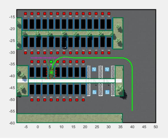
The vehicle tracks the reference path using the MPC controller before switching to the RL controller when the target spot is detected. The vehicle then completes the parking maneuver.
