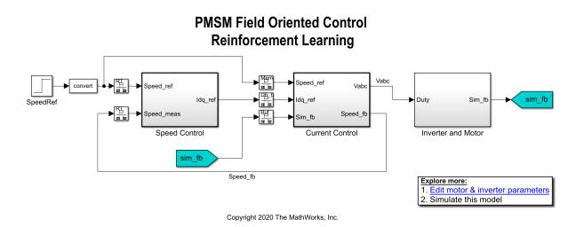
In a linear control version of this example, you can use PI controllers in both the speed and current control loops. An outer-loop PI controller can control the speed while two inner-loop PI controllers control the d-axis and q-axis currents. The overall goal is to track the reference speed in the Speed\_Ref signal. This example uses a reinforcement learning agent to control the currents in the inner control loop while a PI controller controls the outer loop.
