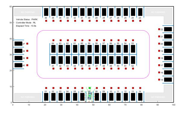
The vehicle reaches the target pose within the specified error tolerances of +/-0.75 m (position) and +/-10 degrees (orientation).
