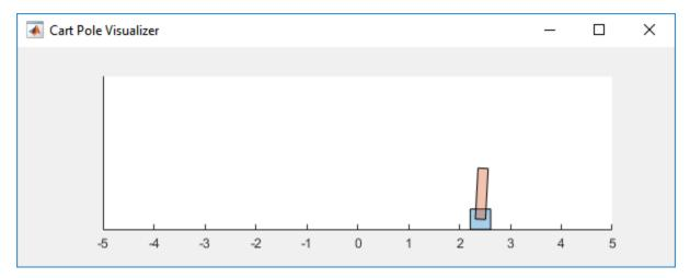
frictionless track. The training goal in this environment is to balance the pole by applying forces (actions) to the prismatic joint.
