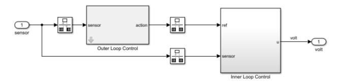
The overall control system consists of two RL Agents in the outer loop computing high level reference angles. The reference angles are sent to a low-level controller that stabilizes the pendulum system by computing the motor voltage. For more information on the controller design and training, see "Train Reinforcement Learning Agents to Control Quanser QUBE Pendulum" on page 5-125.
