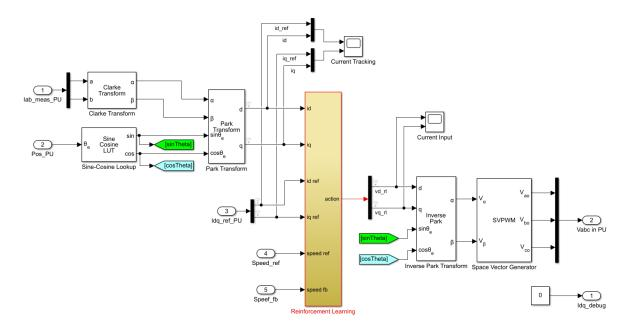
The Reinforcement Learning subsystem contains an **RL** Agent block, the creation of the observation vector, and the reward calculation.
