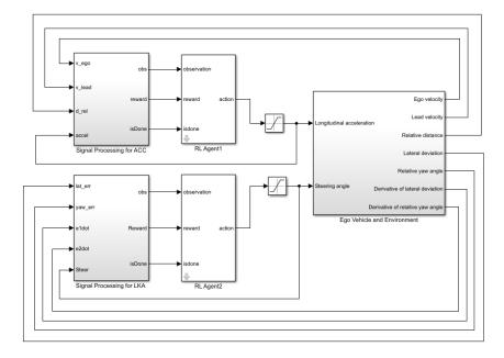
In this model, the two reinforcement learning agents (RL Agent1 and RL Agent2) provide longitudinal acceleration and steering angle signals, respectively.
