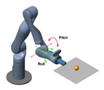
Open the Simulink® model to view the system. The model contains a Kinova Ball Balance subsystem connected to an RL Agent block. The agent applies an action to the robot subsystem and receives the resulting observation, reward, and is-done signals.
