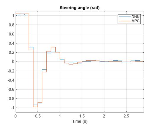
The deep neural network successfully imitates the behavior of the MPC controller. The vehicle state and control action trajectories for the controller and the deep neural network closely align.
