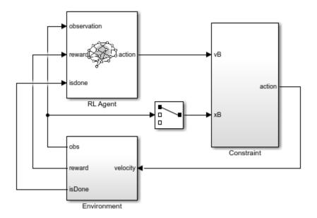
To view the constraint implementation, open the Constraint subsystem. Here, the trained deep neural network approximates  $h(x_k)$ , and the Constraint Enforcement block enforces the constraint function and velocity bounds.
