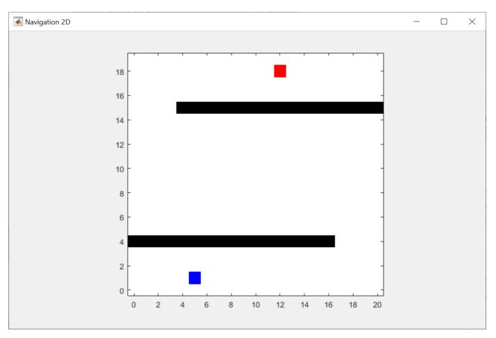
The navigation problem in this example is a goal-conditioned task for which the observation from the environment contains both the goal (navigation target) and the goal measurement (robot position). The observation column vector contains the robot position ( $x_{robot}$ ,  $y_{robot}$ ) and the navigation target
