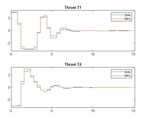
The DAgger neural network successfully imitates the behavior of the NLMPC controller. The flying robot states and control action trajectories for the controller and the DAgger deep neural network closely align. The closed-loop simulation time for the DNN is significantly less than that of the NLMPC controller.
